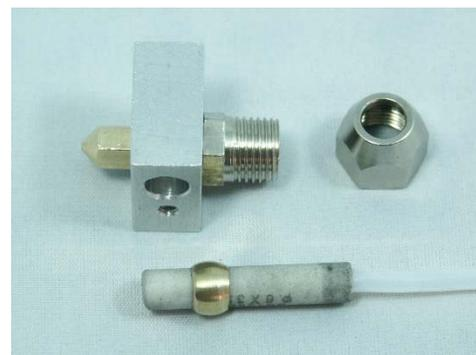
4. Assemble ceramic tube and compression tube fitting. The brass compression ring comes along with the tube fitting is too stiff in this application so obtaining a tight
