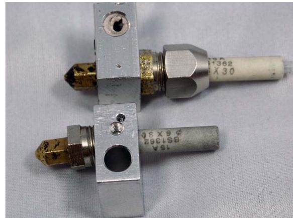
As shown in photo, the lower part is created by drill and tap the heater block with pipe fitting threads so the heater block can act as the compression nut, which further reduces the size and weight of the assembly, however in this case aluminum heater block material is not suitable for compression nut application and initial trail is plagued with oozing, also partially due to poor drill and tap tolerance.
