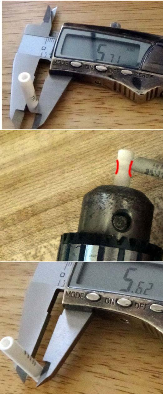
This is an essential step that made this design possible, as to mitigate the loose fitting problem once the hot end heats up. Metal tube fitting's thermal expansion rate is about 0.5% higher than that of ceramic at 250°C, such that the compression ring will lost grip once the hotend heats up. The 2% necked region created in this step ensures that the compression ring will be secured to the ceramic tube at desired working temperature.
